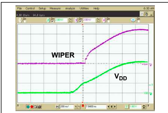
FIGURE 2-15: 2.1 k \Omega – Power-Up Wiper Response Time.
