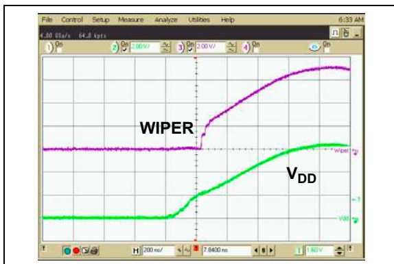
FIGURE 2-52: 50 kΩ – Power-Up Wiper Response Time.
