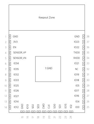
Figure 1: ESP32-WROOM-32 (ESP-WROOM-32) Pin layout
