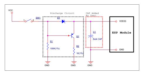
Figure 5: Discharge Circuit for VDD33 Rail
