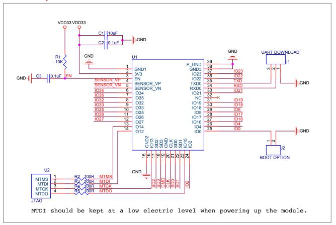
Figure 4: ESP32-WROOM-32 (ESP-WROOM-32) Peripheral Schematics
