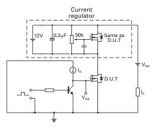
Gate charge test circuit
