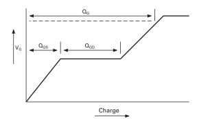
Basic gate charge waveform
