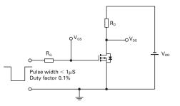
Switching time test circuit
