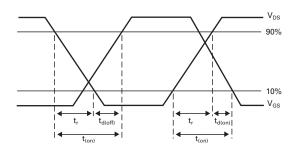
Switching time waveforms
