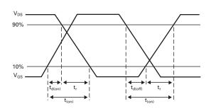
Switching time waveforms
