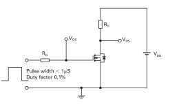
Switching time test circuit
