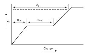
Basic gate charge waveform
