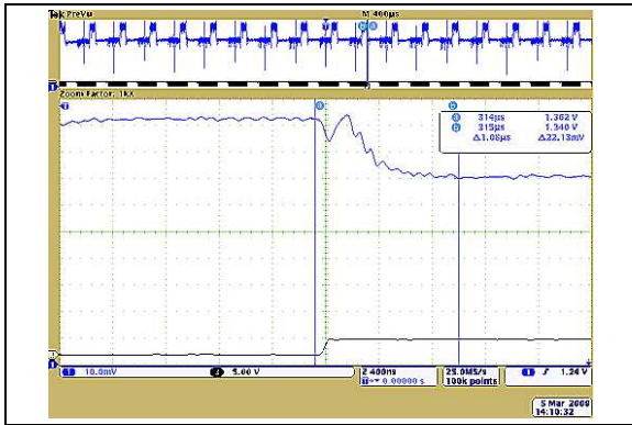
FIGURE 2-16: 5.0 k \Omega : Write Wiper (40h \rightarrow 3Fh) Settling Time ( V_{DD}=2.7\text{V} ).
