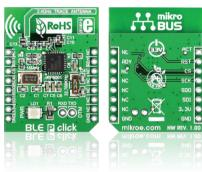
BLE P click<sup>™</sup> is a simple solution for adding a Bluetooth 4.0 (alternatively known as Bluetooth Low Energy) peripheral device to your design. It communicates with the target board through **mikroBUS™** SPI (CS, SCK, MISO, MOSI), INT (RDY) and AN (ACT) lines. Beside the mikroBUS™ socket, BLE P click™ also features additional UART input and output pins (RXD and TXD). These enable you to test the RF parameters of the BLE P's radio design. The board uses a 3.3V power supply only.
