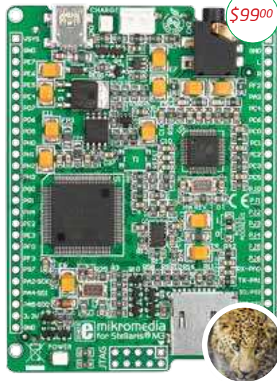
mikromedia for Stellaris M3 (features LM3S9B95)
