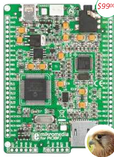
mikromedia for PIC18F (features PIC18F87J50)
