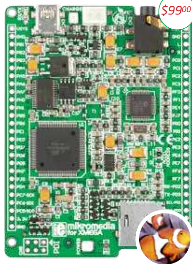
mikromedia for XMEGA (features ATXMEGA128A1)
