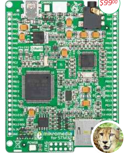
mikromedia for STM32 (features STM32F207VGT6 or STM32F407VGT6)
