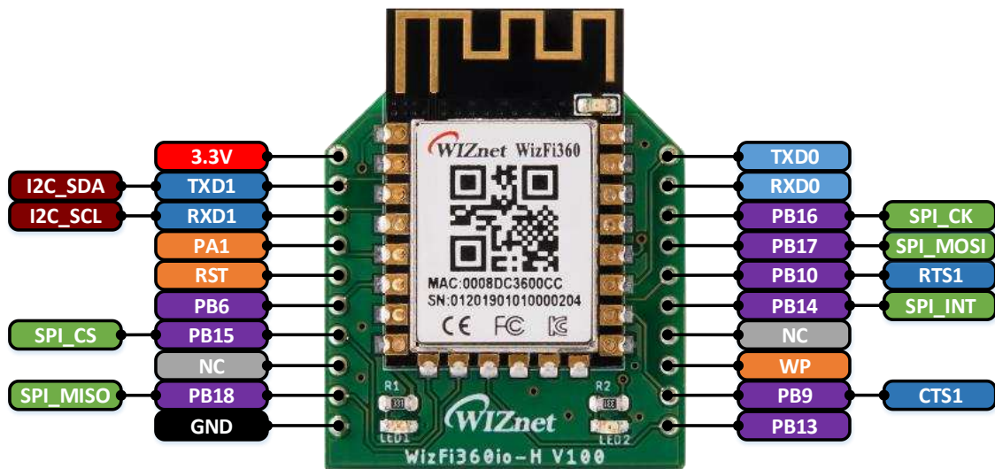
Figure 2. WizFi360io-H Pinout
