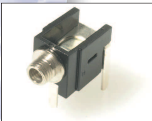
JYO-26 mono switched 2.5mm Jack. Right Angle PCB mounting with ring nut. Thread-less nose version JYO-26A.
