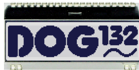
Orientation for 6 o'clock (Bottom View)
