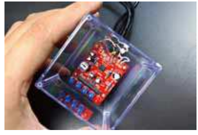
Use tweezers and a magnetic screwdriver to auxiliary install the PCB. First fix one screw without tightening, then install other screws, and finally tighten the screws.
