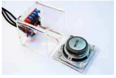
Solder the wires of the loudspeaker, connect the red wire to +, and the transparent wire to-.
