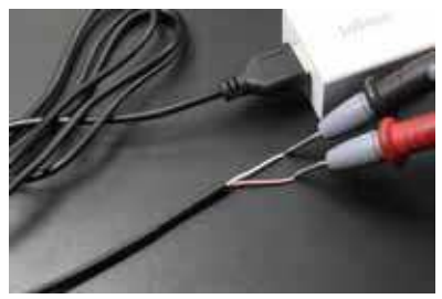
Insert the USB into the USB power supply head, and measure the positive and negative poles of the two wires with the multimeter voltage range.
