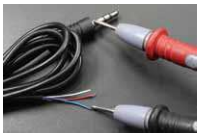
Refer to the circuit schematic diagram and measure the corresponding line of the audio wire.
