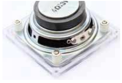
As the picture shows, fix the loudspeaker with nylon posts and screws.
