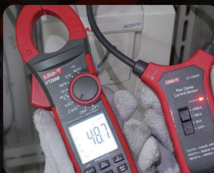
Flexible current probe (optional) to extend the AC current measurement range to 3000A (UT206B/208B)
