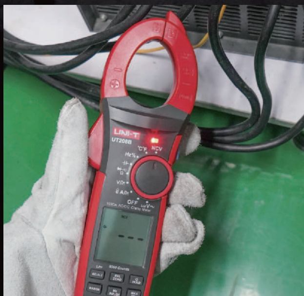
NCV Multi-Segment Display and audio/visual alarm
