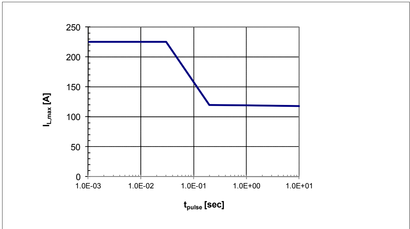
Figure 4 Maximum Single Pulse Current vs. Pulse Time, T_J \leq 150^\circ\text{C} , T_{PIN} = 85^\circ\text{C}
