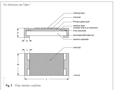
Chip Resistor Surface Mount RC SERIES 0805 (RoHS Compliant)
