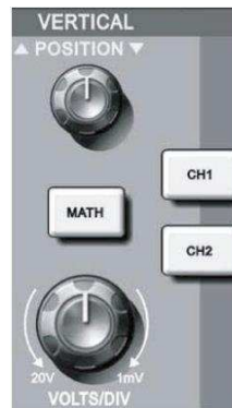
Figure 1-6 Vertical Control Area on the Panel
