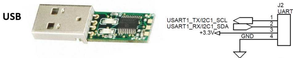
Figure 9. UART TX/RX (3v3 level)
