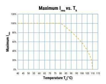
$T_h$  is the maximum ambient temperature surrounding the capacitor or hottest contact point (e.g. tracks), whichever is higher, in the worst operation conditions in °C.
