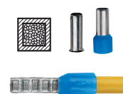
Form of crimping on wire.
