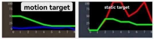
red line:the energy value of each stationary target on the distance door green line:set sensitivity blue line:the energy value of the moving object on each distance gate
