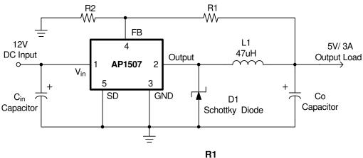
$$V_{OUT} = V_{FB} \times (1 + \frac{R1}{R2})$$
