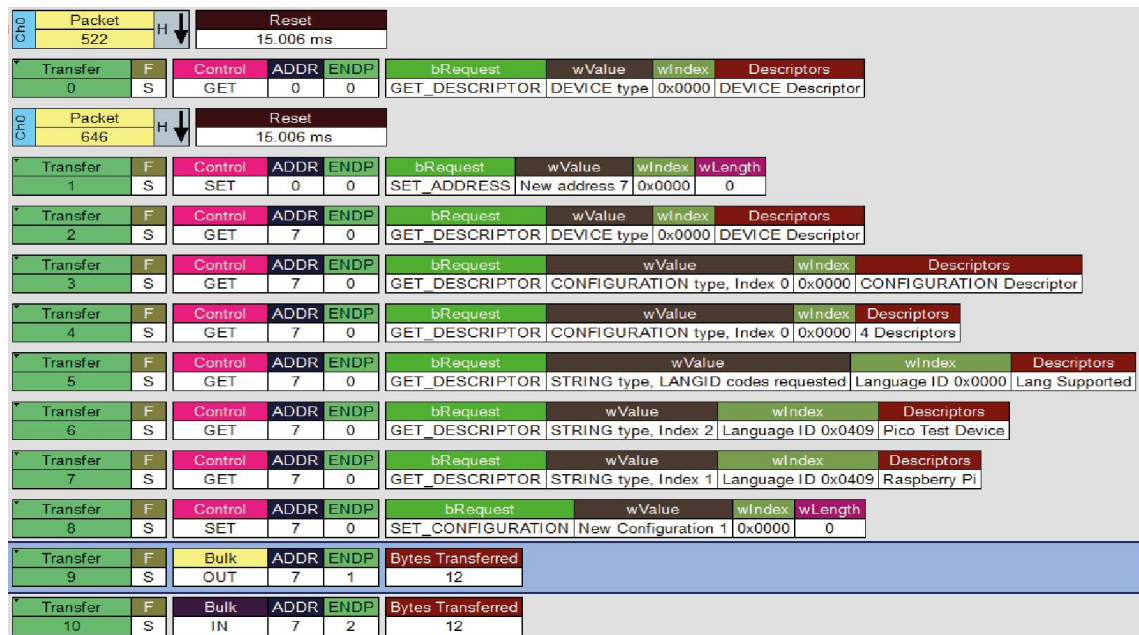
Figure 124. USB analyser trace of the dev_lowlevel USB device example. The control transfers are the device enumeration. The first bulk OUT (out from the host) transfer, highlighted in blue, is the host sending "Hello World" to the device. The second bulk transfer IN (in to the host), is the device returning "Hello World" to the host.
