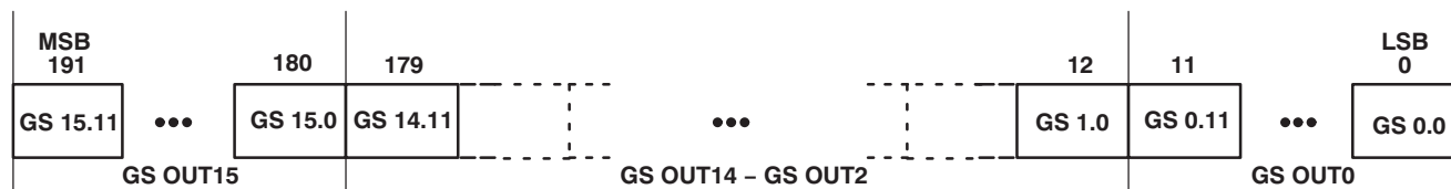
Figure 18. Grayscale Data Packet Format
