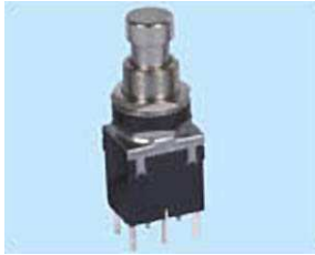
PS24202P ON-ON PS24212P ON-(ON) 4 A 125 VAC; 2 A 250 VAC DPDT 6P (L=14.2, 11.8, 9.8)
