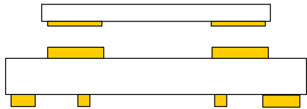
Figure 20. Correct PCB Top Metal Pattern Under Package
