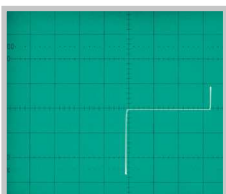
Characteristic of a Z-Diode with Component Test Mode
