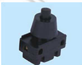
PS17A3 ON-OFF (PBS-17B) 4 A 125 VAC; 2 A 250 VAC
