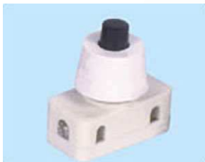
PS17A ON-OFF 4 A 125 VAC; 2 A 250 VAC
