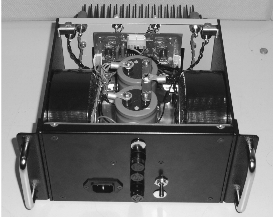
Figure 1. Complete LM4702-Based 100W/Channel High-Fidelity Power Amplifier
