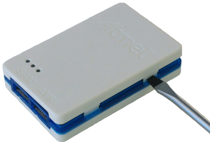
Figure 2-13. Opening the Atmel-ICE (2)
