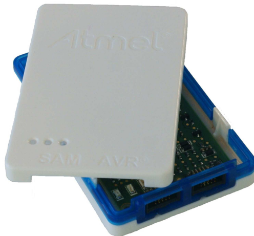
Figure 2-14. Opening the Atmel-ICE(3)
