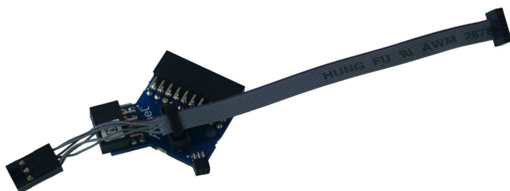
Figure 2-9. Atmel-ICE Cable Connection
