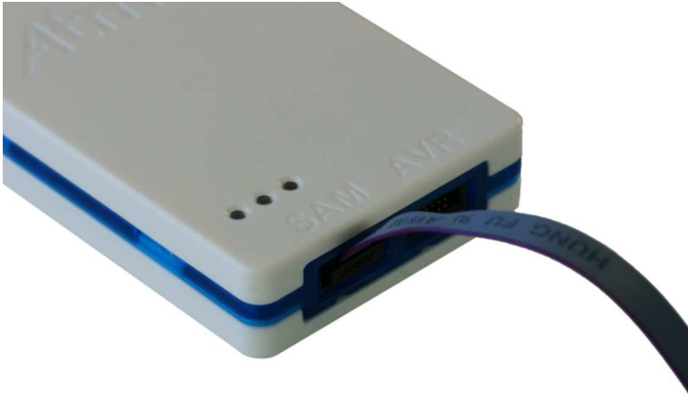
Figure 2-11. Atmel-ICE SAM Probe Connection
