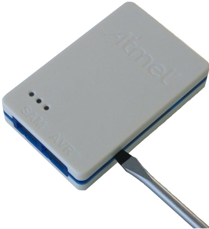
Figure 2-13. Opening the Atmel-ICE (2)
