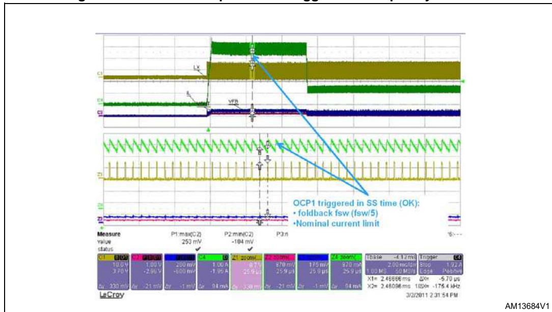
Figure 23. Over current protection triggers the frequency foldback
